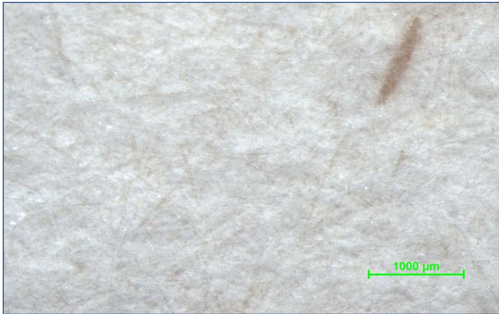
Figure 3: Fresh fibre board under transmission light microscopy
