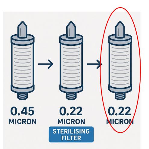
8.80: Due to the potential additional risks<sup>\*)</sup> of a sterile filtration process, as compared with other sterilisation processes, an additional filtration through a sterile sterilising grade filter, as close to the point of fill as possible, should be considered as part of an overall CCS.
