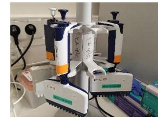
Multichannel pipette or Stepper
