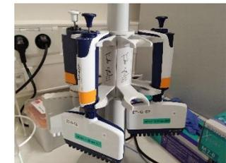
Multichannel pipette or Stepper
