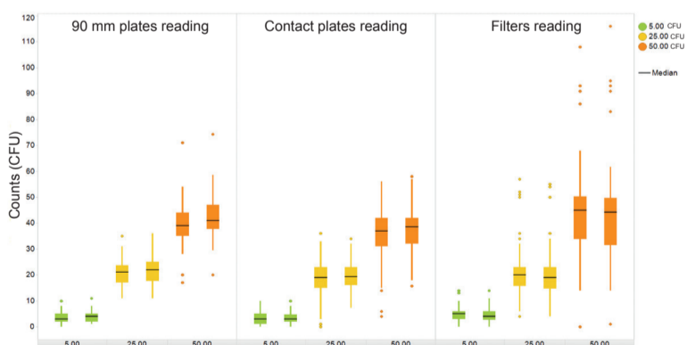
Figure 5: Boxplots of microorganisms counts obtained with EviSight™ compact (left side of the pair) and manually (right side of the pair)
